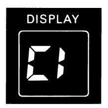
This flashing code tells you to check the automatic icemaker. Ice clumps in the storage bin may have stalled the icemaker. Follow corrective measures described on page 13. If water supply to the icemaker is not connected or not turned on, make sure manual icemaker switch is in the OFF position (see page 11). Code stops flashing when problem is corrected or STATUS CHECK-RESET pad is touched.
